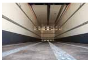
The pneumatic roller floor
